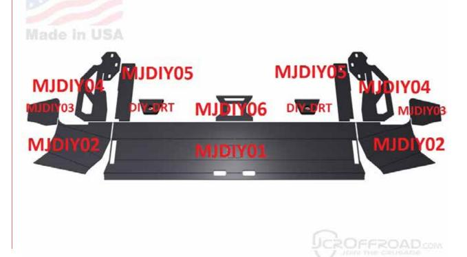
The first piece you will want to bend will be the (MJDIYO1) Bumper Face / Center Section. You will be bending 3 angles. It doesn't matter which side you make the front face.
