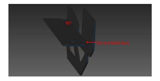
5 With everything bent, it's time to start tacking everything together. It's best to weld and grind the shell of the bumper without the Dring tabs or Bumper mounts welded on first.
