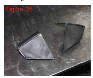
Setting the Center Section on your work table, line up and tack weld the wings in place.
