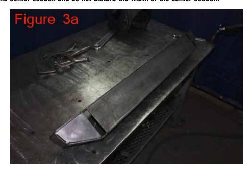
4 With the bumper tacked together, it is now time to fully weld the bumper together. We recommend welding the back side first.
