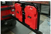
13. Adjust mounts/bracket so that cans are sitting on the tire carrier base. Tighten bracket to carrier and then can mounts to bracket. Tighten RotopaX handles until they lock in place.
