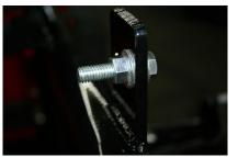
10. If installing a Hi-Lift jack, open tire carrier and lock in place. Using 7/16" x 1 1/2" bolts, washers, and nuts, assemble in following order: bolt with washer from outside pointing inward, washer then nut on inside of bracket,
