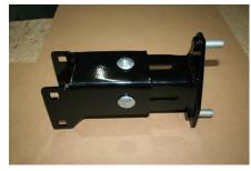
placement of tire mount on the carrier center support, there will likely be some trial and error. To get an idea, (and knowing your tire dimensions) you can measure the height off the bumper. A stock tire will have the mount sitting lower while a larger diameter will require it higher. Insert four
